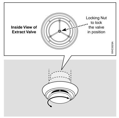
**EV100** Adjust Ceiling Extract Valve for Bathroom etc
